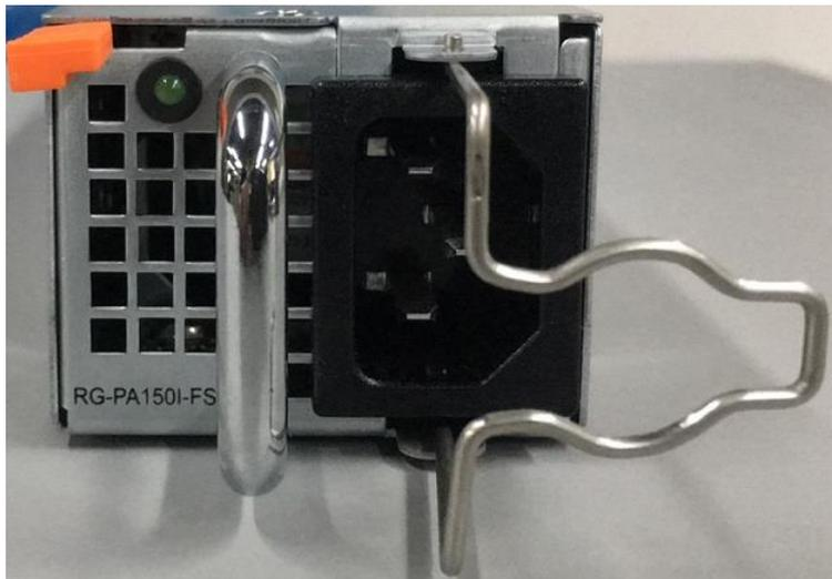
RG-PA150I-FS is an AC power module with AC power input and provides 12 V voltage to the entire RG-NBS6002 system. The front panel of the power supply provides a three-pin power socket, which is connected with a standard 10 A power cord.
