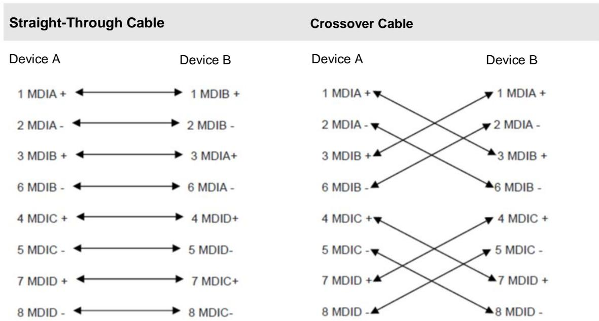
Table 7-2 Definition of Pin Signal Concerning the 100BASE-TX/10BASE-T Port
